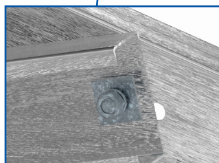
Bolt M12 with 2 Square Washer
